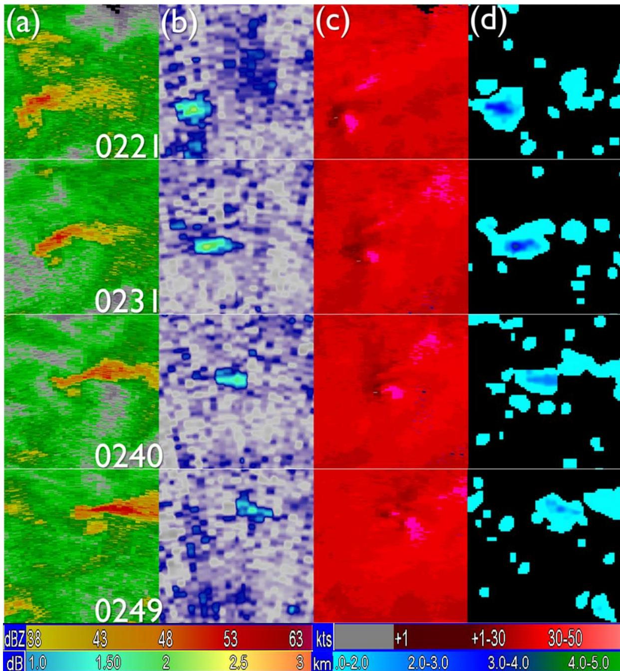
Fig. 3: a) 0.5° reflectivity  $Z_H$  PPI (scale upper-left), b) 5-km AGL differential reflectivity  $Z_{DR}$  CAPPI (scale lower-left), c) 0.5° base velocity (scale upper-right), and d)  $Z_{DR}$  column algorithm output (scale lower-right) from KBMX on 29 April 2014. A tornado developed from this supercell at 0239 UTC. Note the decrease in  $Z_{DR}$  column height after 0231 UTC.
