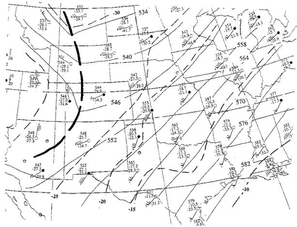
FIG. 4. The 500-hPa analysis valid 1200 UTC 1 Mar 1997. Solid lines represent geopotential heights in dm with dashed lines temperatures in  $^{\circ}C$ . For this plot, numbers from top to bottom are height (in dm), temperature, and dewpoint, respectively. A half wind barb is  $5 m s^{-1}$ , full barb  $10 m s^{-1}$ , and pendant is  $25 m s^{-1}$ .
