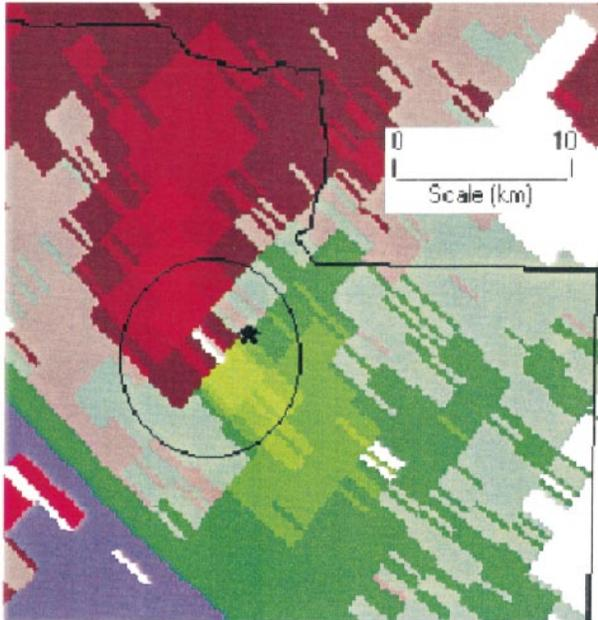
FIG. 22. KLZK storm-relative velocity map image ( $0.5^\circ$  elevation scan) for 2042 UTC at the time an F4 tornado is entering Arkadelphia. Area enclosed in open circle depicts circulation core of supercell A. Star shows approximate location of the center of Arkadelphia. Green- and red-shaded areas indicate radial velocities toward and away from the radar, respectively. Lightest shades of red and green denote speeds greater than  $25 \text{ m s}^{-1}$ . See text for further details.
